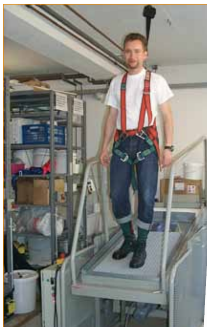
The slip-resistance test for Excellent Systems tiles and ramps was performed by the German testing institute FGK.
